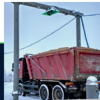
3D laser scanner measures the volume in the truck.
